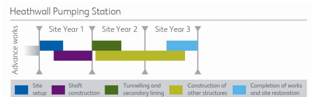
Figure K.6 Construction duration
