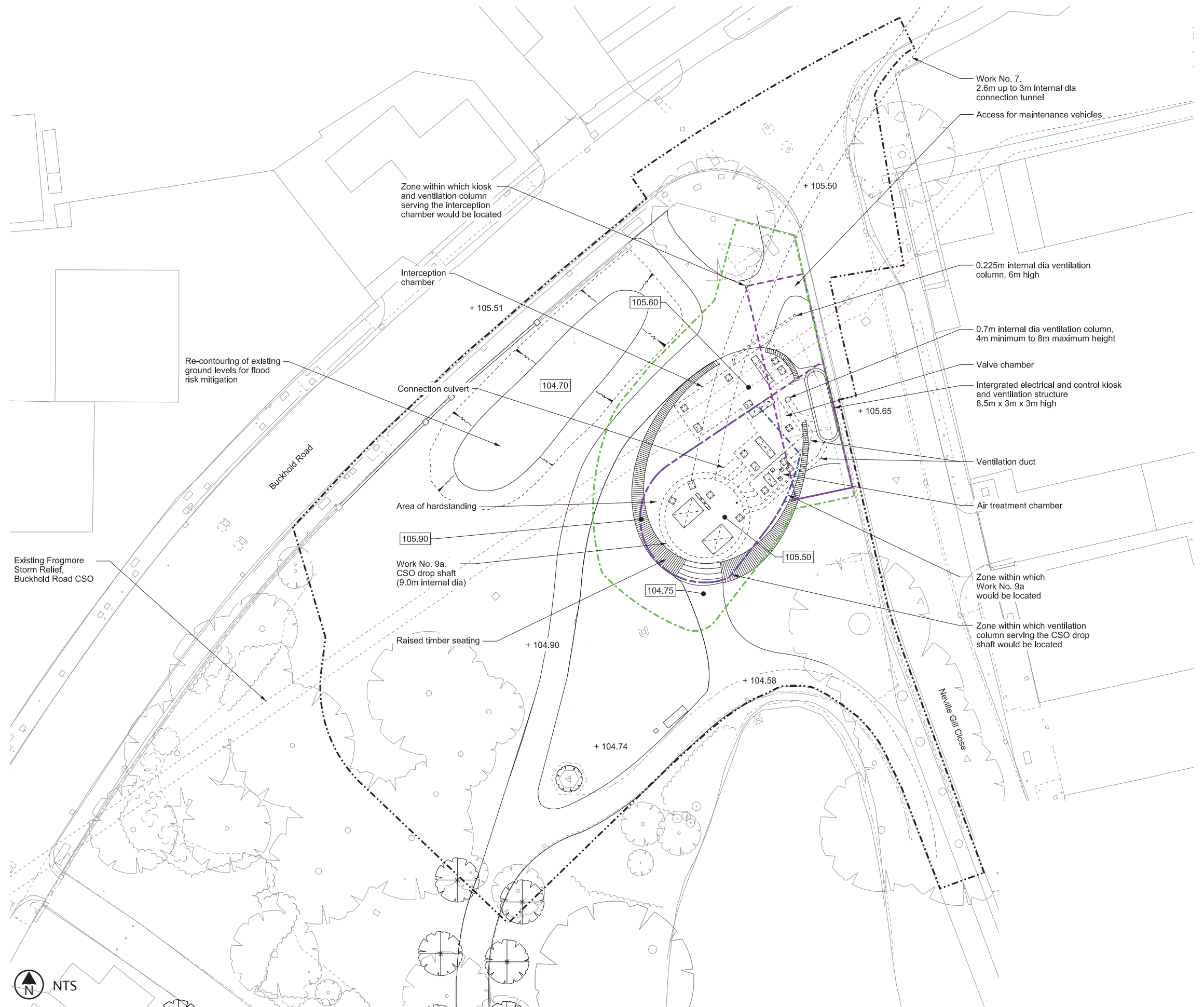
Figure 11.57: Permanent works layout- refer to Permanent works layout in the Book of Plans
