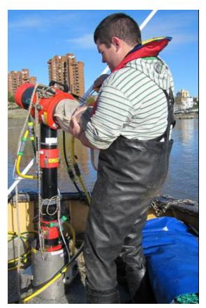
Vol 3 Plate C.42 Airlift sampler (main unit)
