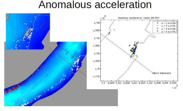
The customised graph on right highlights the position of any anomalously high situations of acceleration between steps 481-500 (~3 hours). The viewer sections on left show typical views of a single step during this time (white being temporary works fish and developments in this case) – some of which get caught between bridge pier and proposed works.
