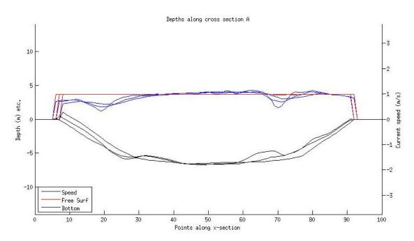
C.2.104 Vol 3 Plate C.17 shows how the current speed drops close to the bridge piers.
