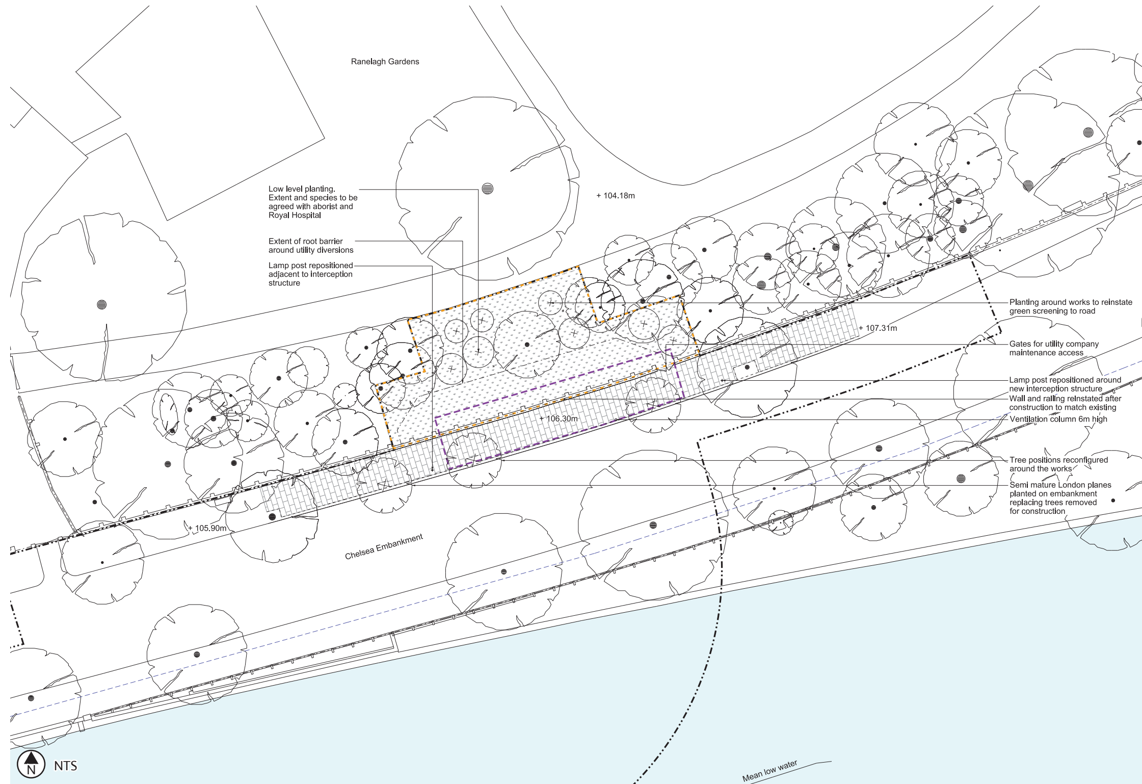
Figure 15.34: Proposed landscape reinstatement works over the connection to the northern Low Level Sewer No 1 - refer to Proposed landscape plan sheet 2 of 2 in the Book of Plans
