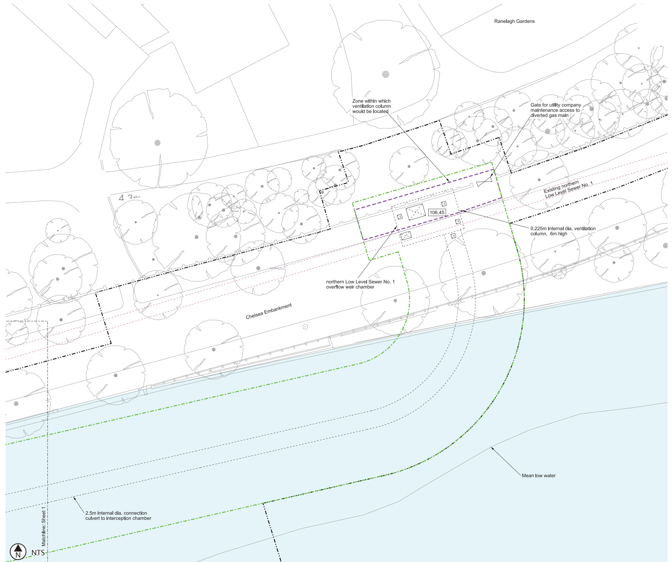
Figure 15.66: Proposed northern Low Level Sewer No.1 connection - refer to Permanent works layout sheet 2 of 2 in the Book of Plans
