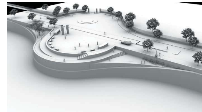
Figure 15.29: Design development study model showing how pedestrian access to lower level could be achieved
