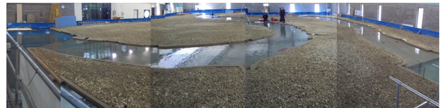
Figure 5.26: Photograph of physical model of the River Thames at HR Wallingford
