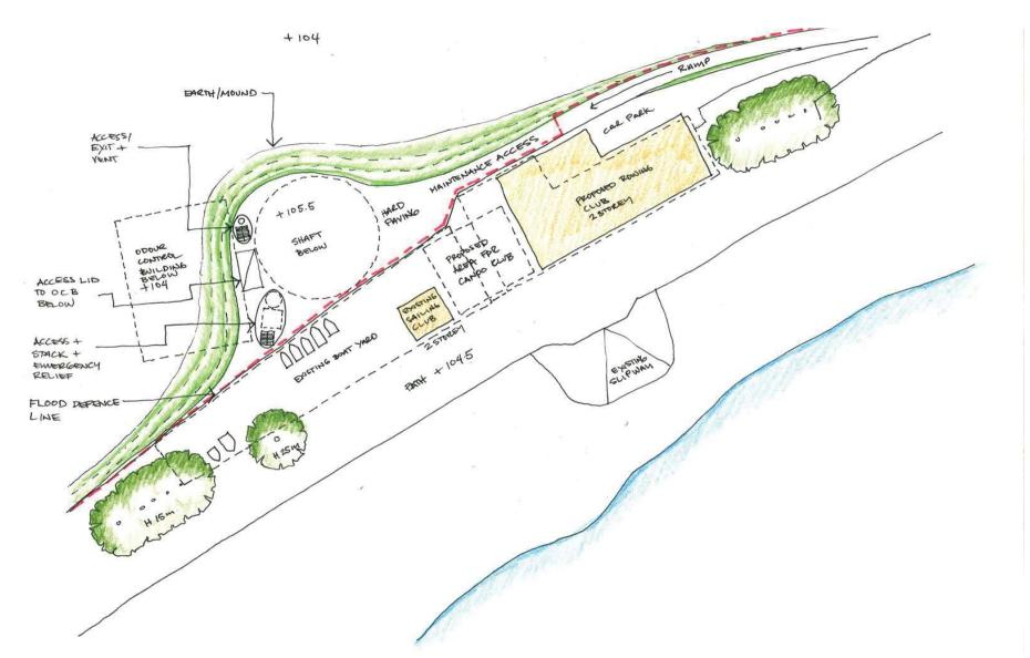
Figure 8.20: Design development diagram showing how the impact of the main tunnel works could be minimised
