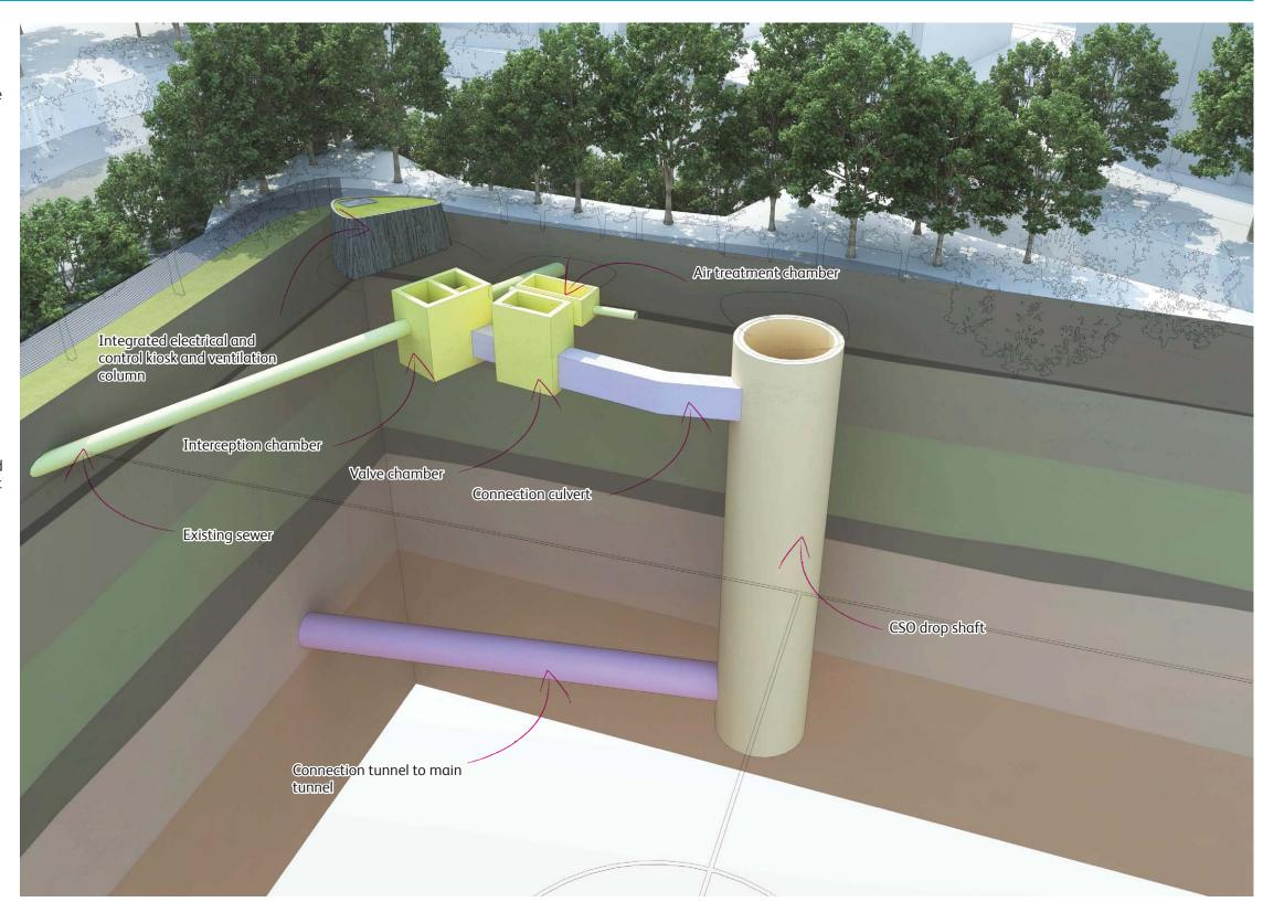
Figure 8.29: Functional components diagram: below ground view
