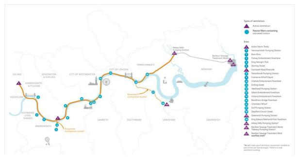
Figure 6.2 Location of active ventilation plant and passive filters
