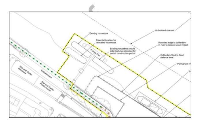
Figure 6.1 Annotated plan of proposed barge relocation
