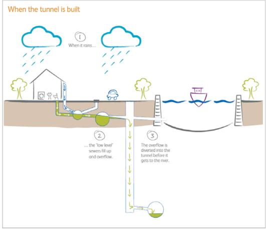
Figure 2.3 When the project is built
