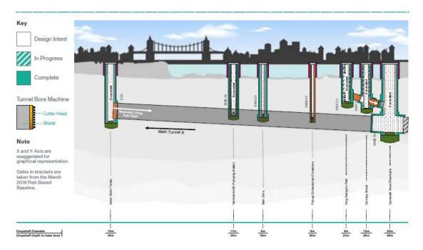
The west team saw the successful completion of tunnelling in September 2020 with Tunnel Boring Machine (TBM) Rachel safely arriving at Acton after starting her 7km journey from Carnwath Road in May 2019. The 1.1km Frogmore connection tunnel was also completed by TBM Charlotte in July 2020. Both TBMs were safely removed from site to be refurbished for future projects.
