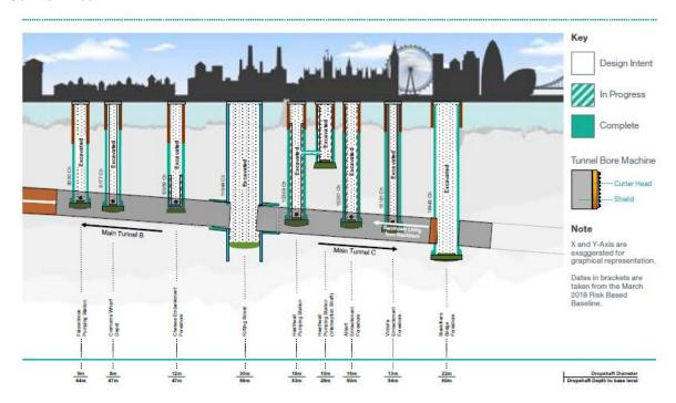
TBM Ursula broke through into the shaft at Tideway's Chambers Wharf site in November 2020, marking the safe completion of the Central section of the main tunnel which stretches from Fulham to Bermondsey. This 12.6km stretch of tunnel was constructed by two TBMs tunnelling in different directions from the shaft at Kirtling Street. Since the completion of tunnelling the team have started casting the concrete secondary lining in the westbound stretch of tunnel.
