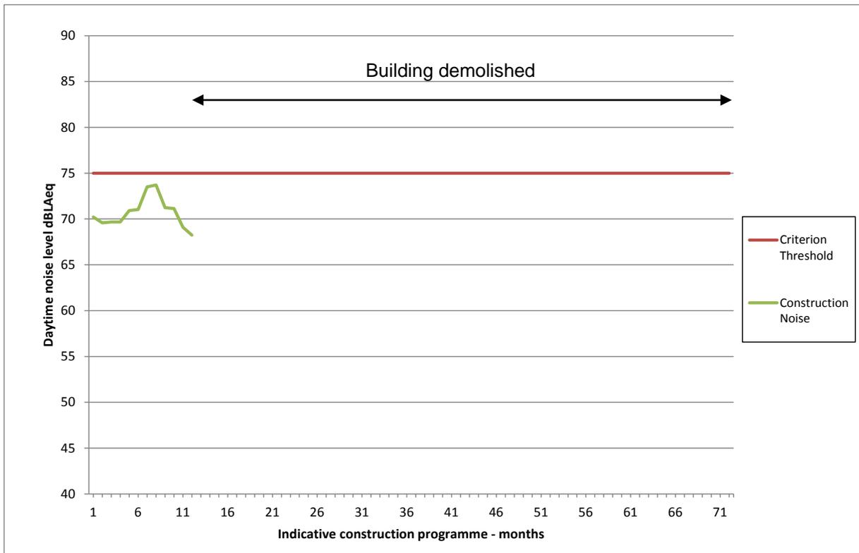
**Vol 14 Plate G.14 Average monthly daytime noise level over duration of construction – Battersea Power Station, Block PS (KS9)**
