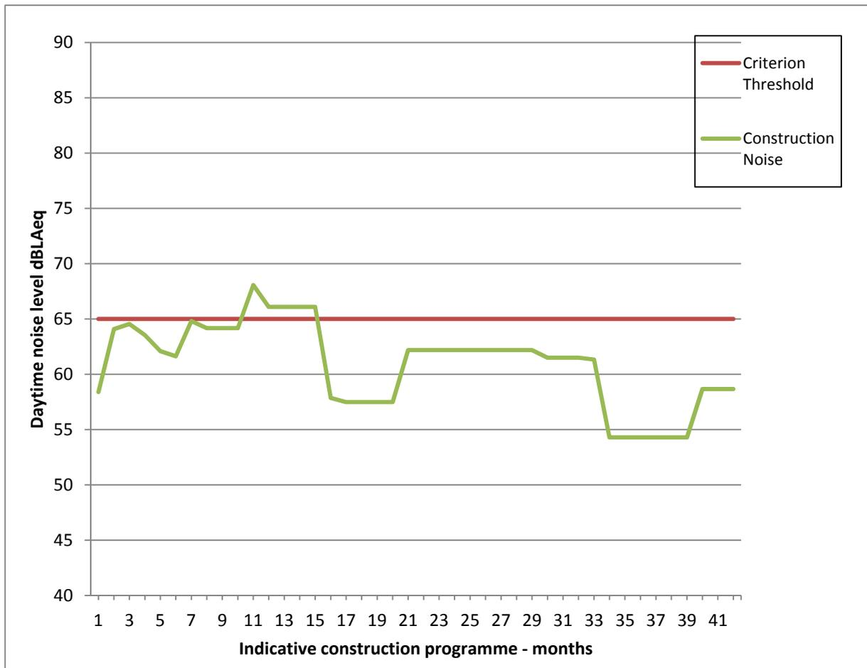
**Plate G.6 Average monthly daytime noise level over duration of construction – Shadwell Basin Outdoor Centre (KE2)**
