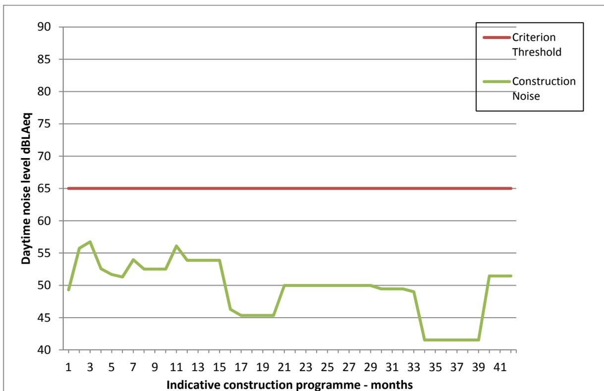
**Plate G.9 Average monthly daytime noise level over duration of construction – 35 Peartree Lane (KE5)**
