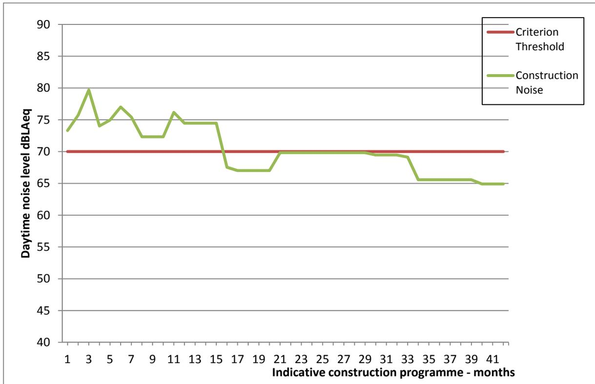
**Plate G.14 Average monthly daytime noise level over duration of construction – Abbotshade Road (KE10)**
