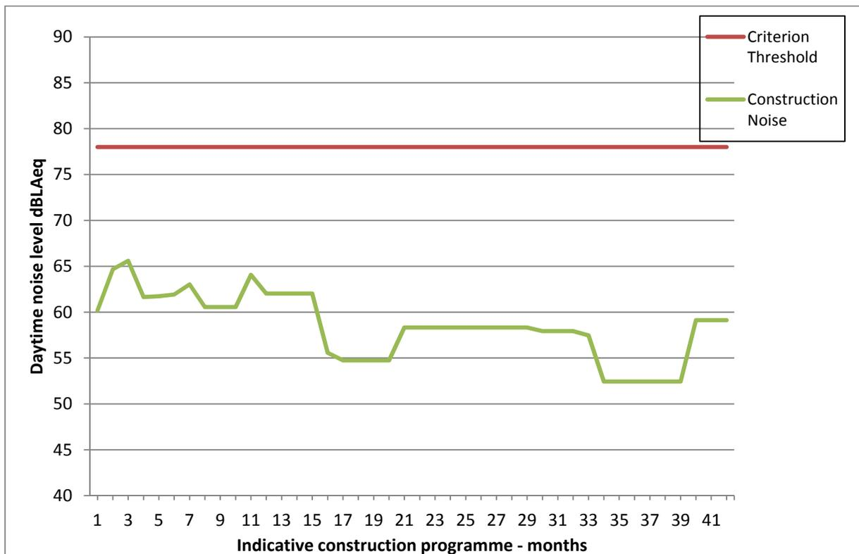
**Plate G.11 Average monthly daytime noise level over duration of construction – Free Trade Wharf North (KE7)**
