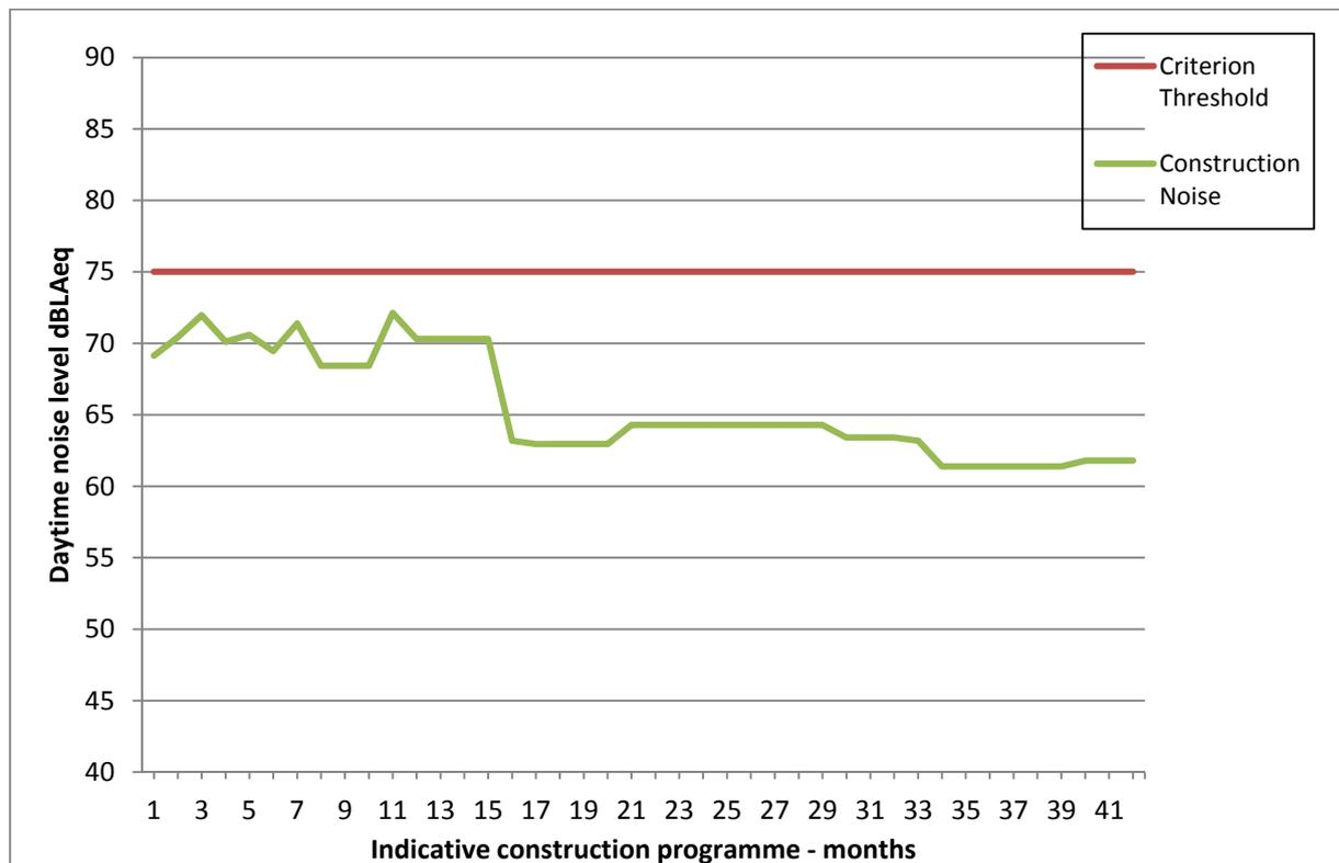
**Plate G.13 Average monthly daytime noise level over duration of construction - Free Trade Wharf South (KE9)**
