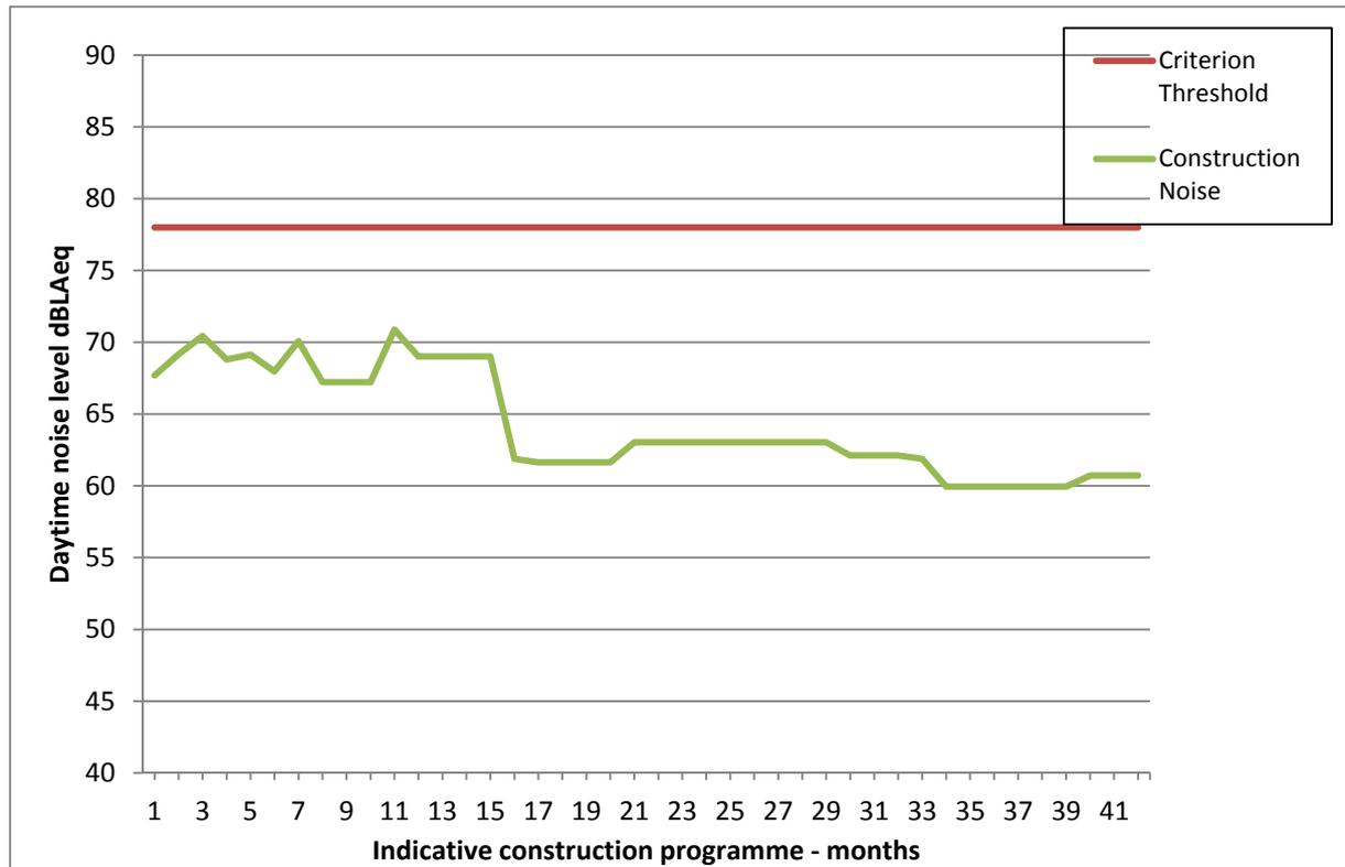
**Plate G.12 Average monthly daytime noise level over duration of construction - Free Trade Wharf Middle (KE8)**
