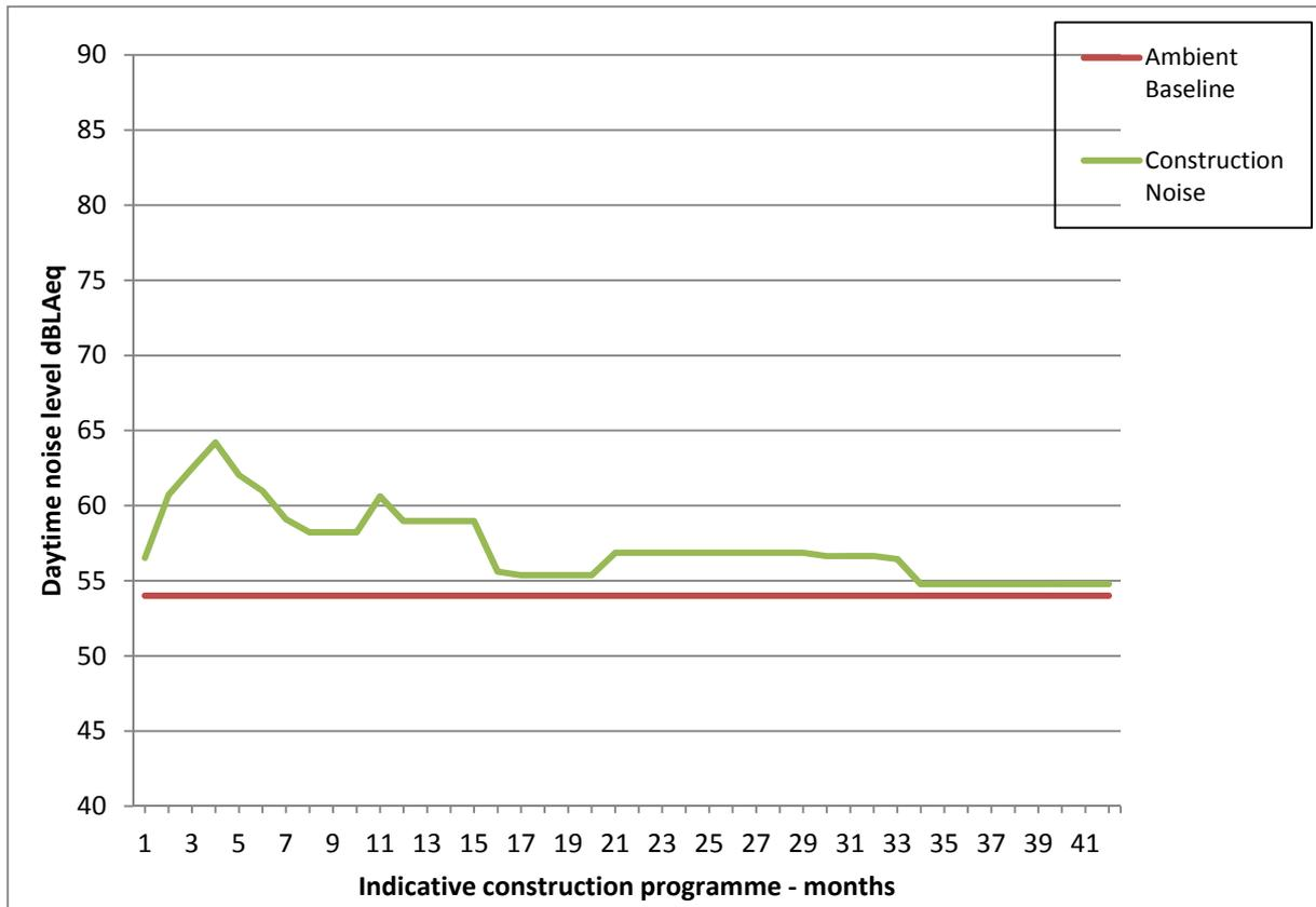
**Plate G.7 Average monthly daytime noise level over duration of construction – Pier Hear Prep. School (KE3)**
