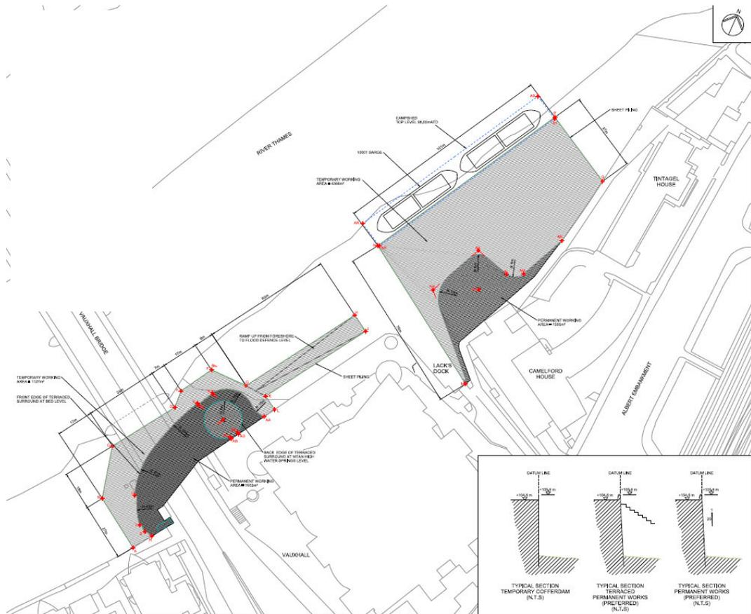
**Figure 11-1 Plan of proposed works at Albert Embankment**
