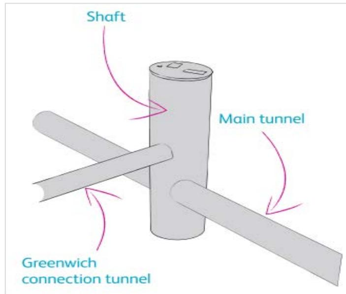
2.2.5 It is proposed that the Chambers Wharf site would operate as a main tunnel drive and reception site and a connection tunnel reception site. The cofferdam and site working area would accommodate the following:
