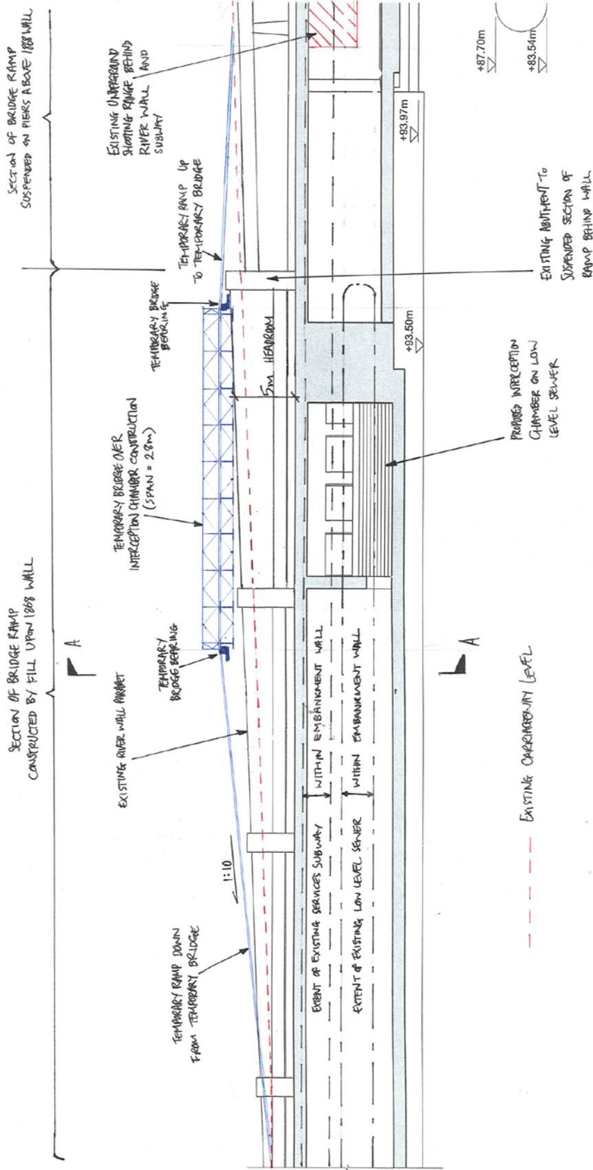
ELEVATION SHOWING TEMPORARY BRIDGE OVER LOW LEVEL SEWER INTERCEPTION CHAMBER
