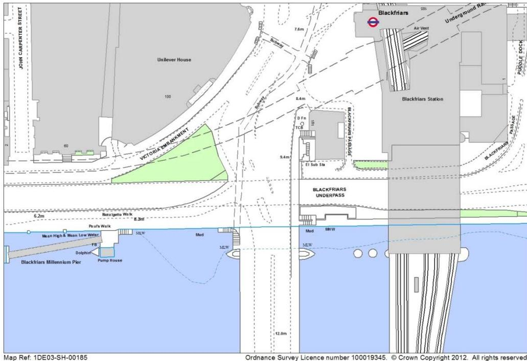
F.2.5 As part of these works, the gas mains were diverted for a short length, and a new service subway was constructed to follow the line of the new river wall. As a result, there is a short length of the sewer that does not have the gas mains over the top of it, located in the infilled section of the ramp (as shown on Plate F.4
