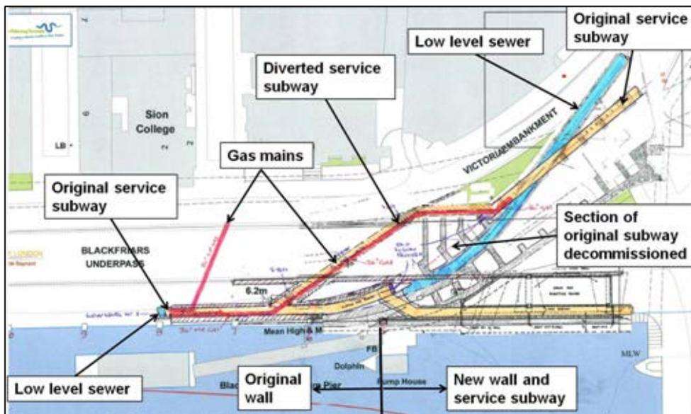
F.2.6 There are two options for making a connection to the low level sewer as illustrated in Plate F.5:
