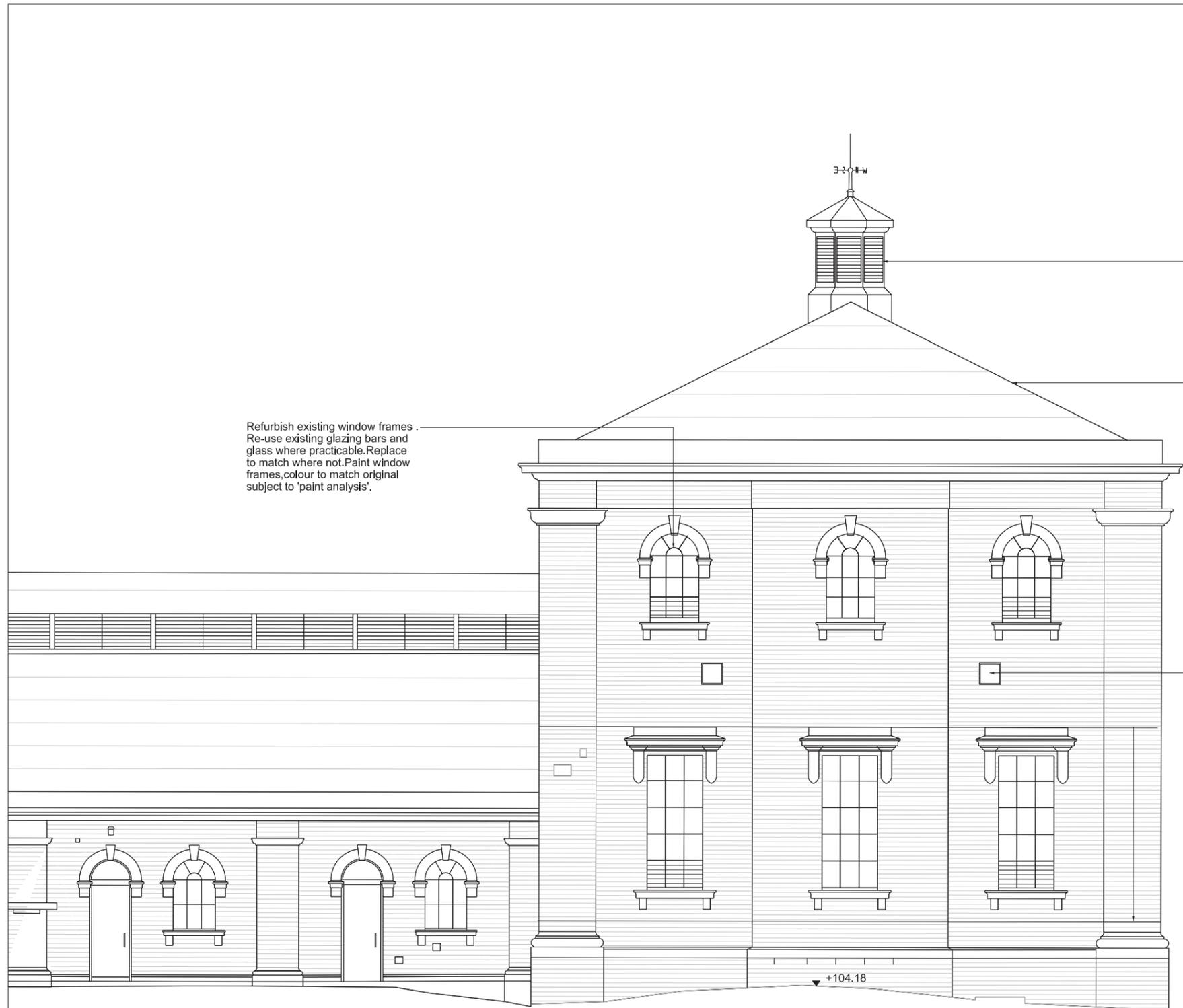
Refurbish existing window frames. Re-use existing glazing bars and glass where practicable. Replace to match where not. Paint window frames, colour to match original subject to 'paint analysis'.
