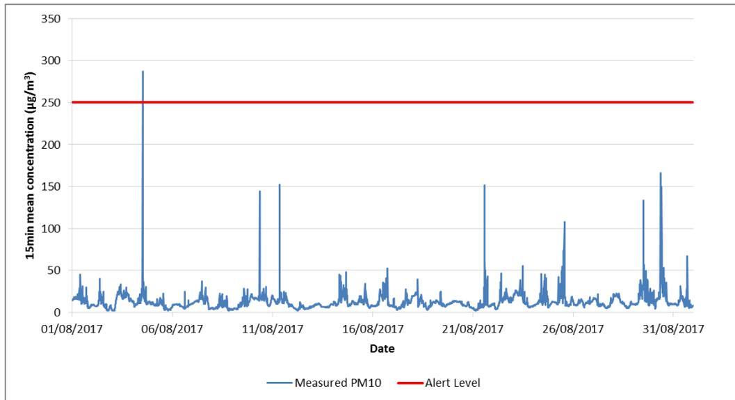
Figure 3 Graph of 15-min PM<sub>10</sub> Concentrations at CARRR/AA/3: August 2017
