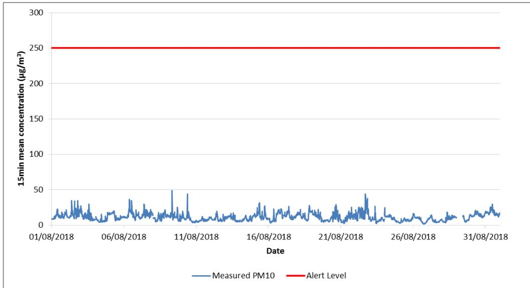
**Figure 2 Graph of 15-min PM<sub>10</sub> Concentrations at CARRR/AA/2: August 2018**
