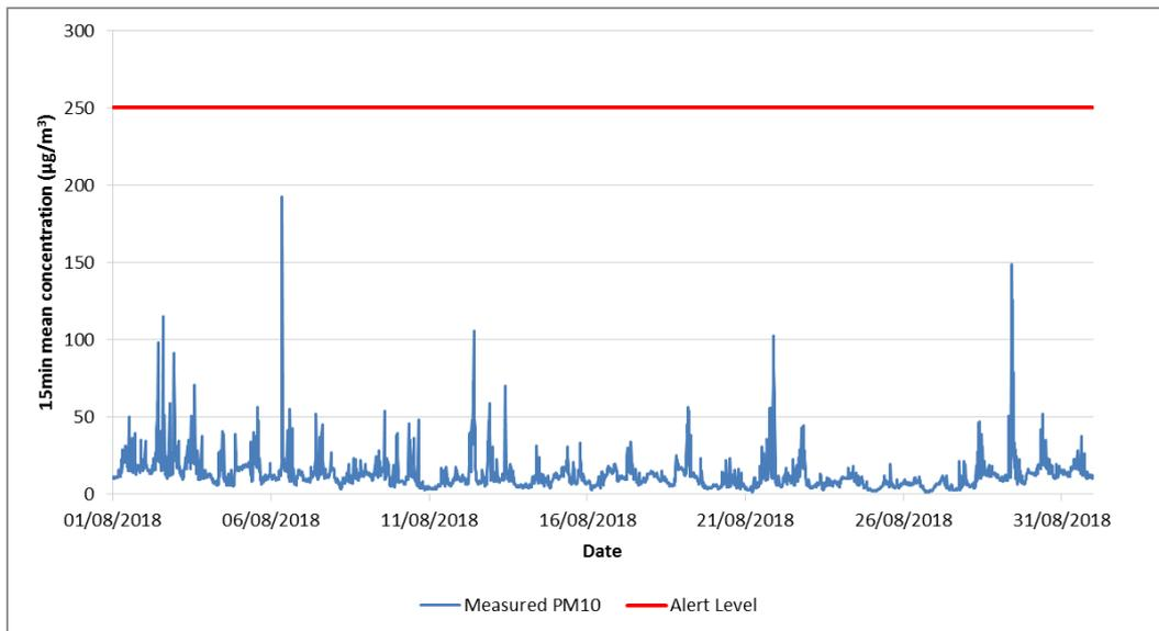
**Figure 3 Graph of 15-min PM<sub>10</sub> Concentrations at CARRR/AA/3: August 2018**
