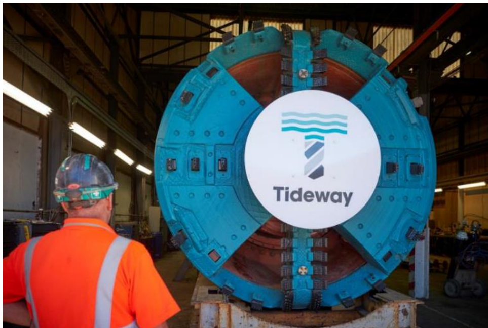
TBM Charlotte undergoing tests at Morgan Sindall, Staffordshire
