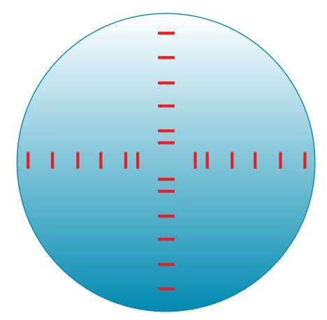
In each row, the cutter disks are the following distances from the centre: 0.5m, 1.0m, 1.5m, 2.5m, 3.5m, 4m
