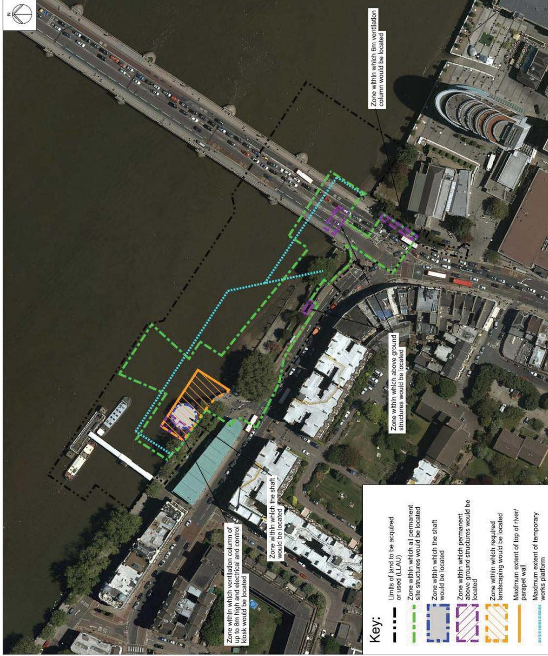
Figure 9.5 Schematic layout at the Putney Embankment Foreshore site
