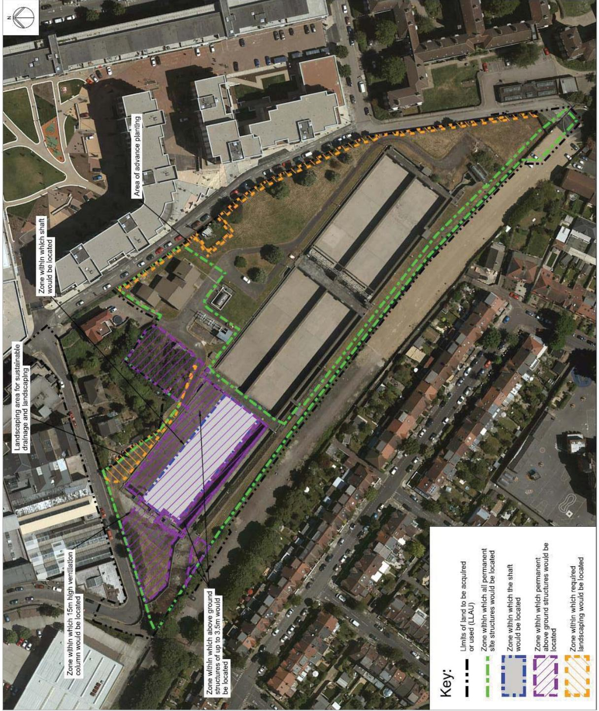
Figure 6.5 Schematic layout of Acton Storm Tanks site
