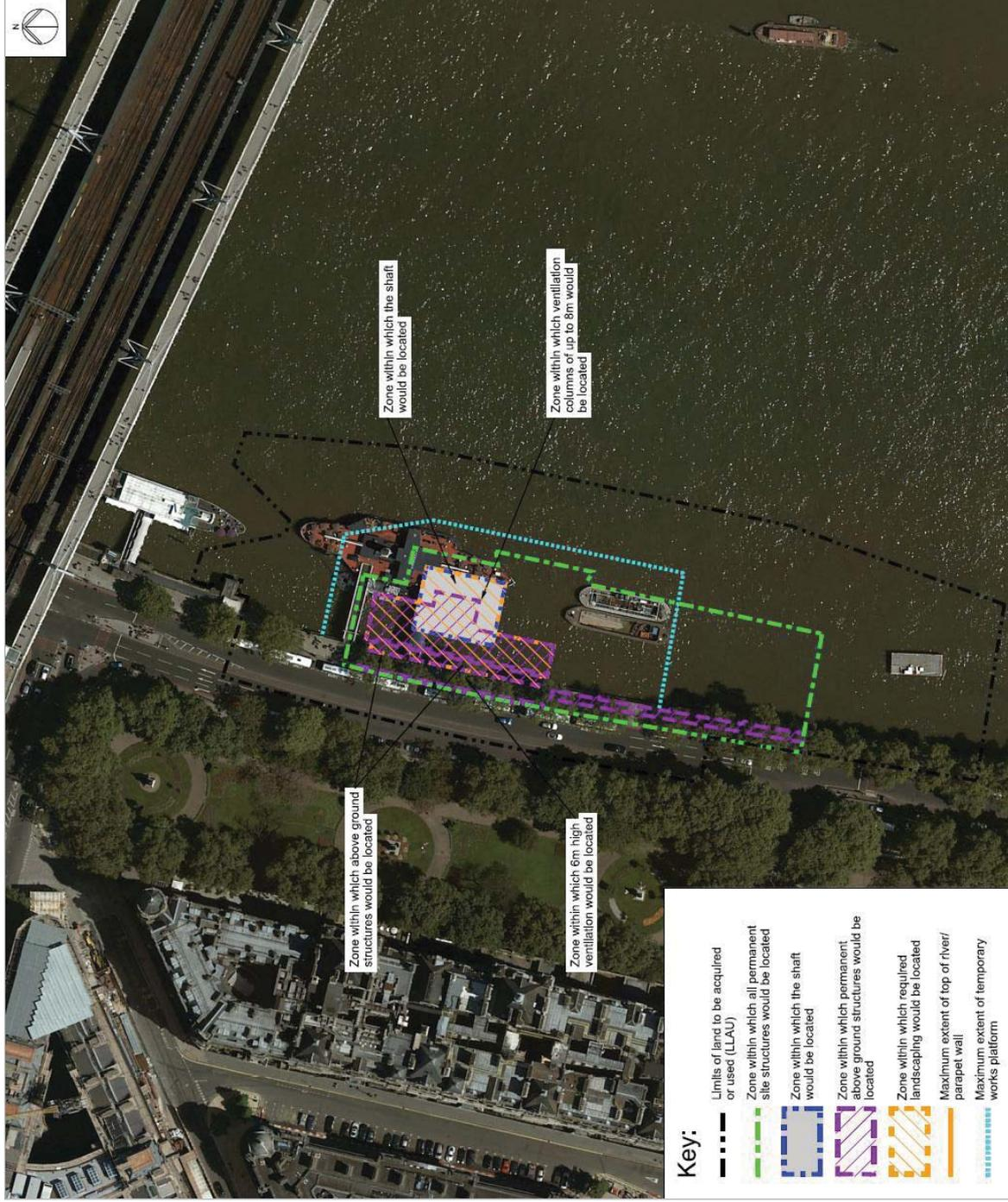
Figure 19.5 Schematic layout at the Victoria Embankment Foreshore site
