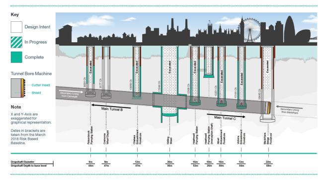
The Central team are working across all eight construction sites, each of which have started or completed excavating their shaft structure. In total, there are nine shafts in Central with two at Heathwall Pumping
