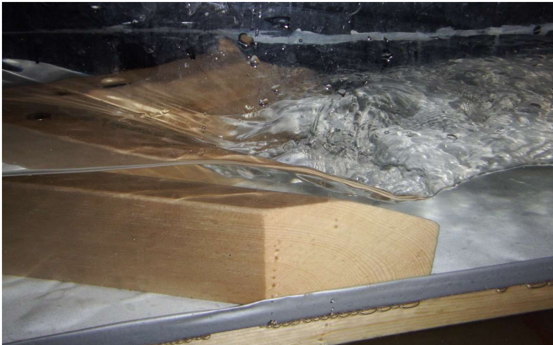
Figure 26 Aerodynamically chamfered object in fast flow. This object was relatively uncomfortable for fish to pass apparently due to the sheet of high speed laminar flow over the object and the centrally concentrated turbulent wake. The laminar layer should be viewed in contrast to the wedge shaped flow pattern produced by the square edged object in Figure 7.
