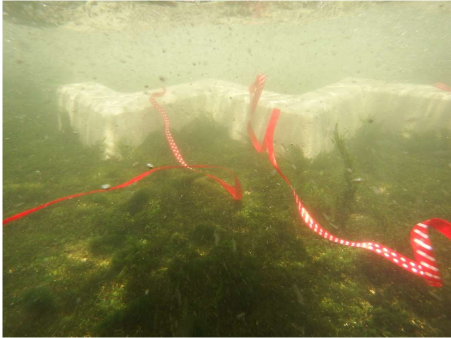
Figure 29 Structure placed on artificial hard substrate in River Test with ribbons used to visualise turbulent wakes of structures
