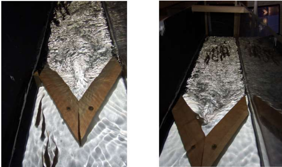
Figure 25 Difference in turbulent wakes of two chevron shaped objects. The object on the left has aerodynamic chamfered downstream edges whereas on the right all the edges are square. The wake of the left hand shape is appreciably more concentrated in the centre. The surface appearance of the water is enhanced through the use of standard flash photography.
