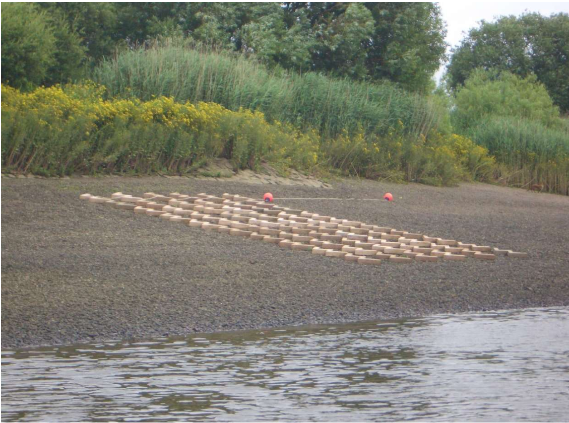
Figure 3: Sixty micromeasures structures laid out at the experimental site on the foreshore of Chiswick Eyot, River Thames.
