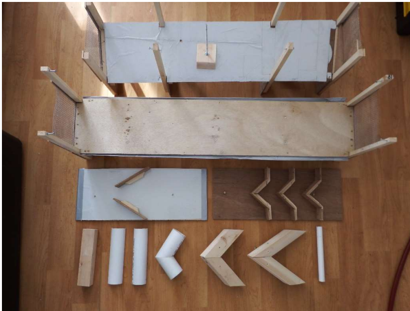
Figure 19 Some examples of the experimental equipment. This collection includes level and inclined planes, turbulence generators, basic shapes, and fish pass type structures
